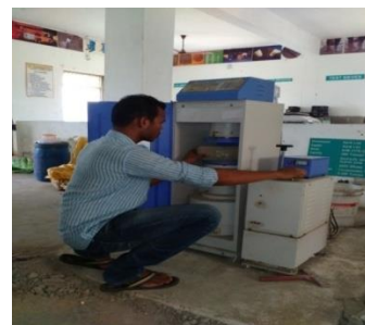
Figure 3.4 Testing of compressive strength
