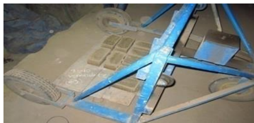
Figure 3.3 Casting of Bricks
